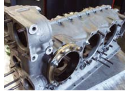
Zeppelin repairs free of distortion finished aluminium components with the aluminium DC-welding process.
