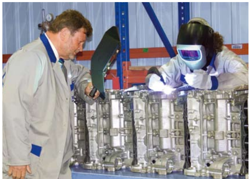
Repair on motor housings – welded without preheating, cracks worked out and fully welded. Advantage: no critical deviations at fits or mechanically machined surfaces after welding.
