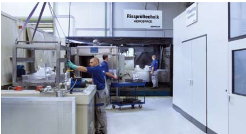
By means of the crack inspection procedures “penetrant inspection” and “magnetic particle inspection” all cracks are detected on ferromagnetic and non-ferromagnetic components.
