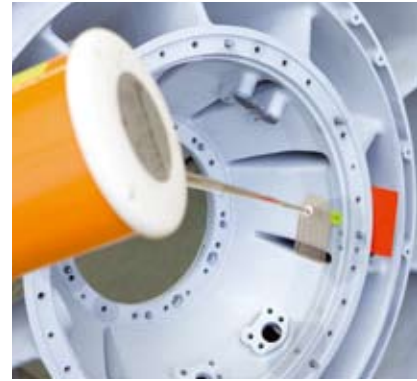
X-ray on aeronautical components by means of a 160 kV tube (picture above).
